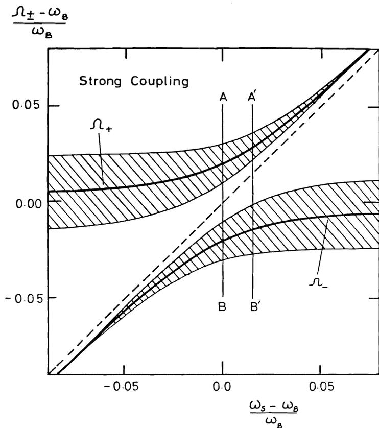
FIG.8(a): Typical dispersion curves for normal modes in the strong coupling limit
