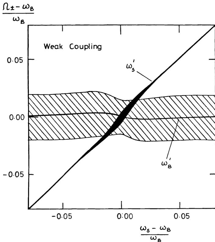
FIG.8(b): Typical dispersion curves for normal modes in low coupling limit
