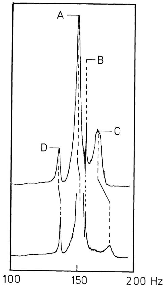
FIG.10:  $n=2$  C-string resonances on a cello, midway between two strongly coupled structural resonances. An additional mass has been placed on the belly for the upper set of measurements.
