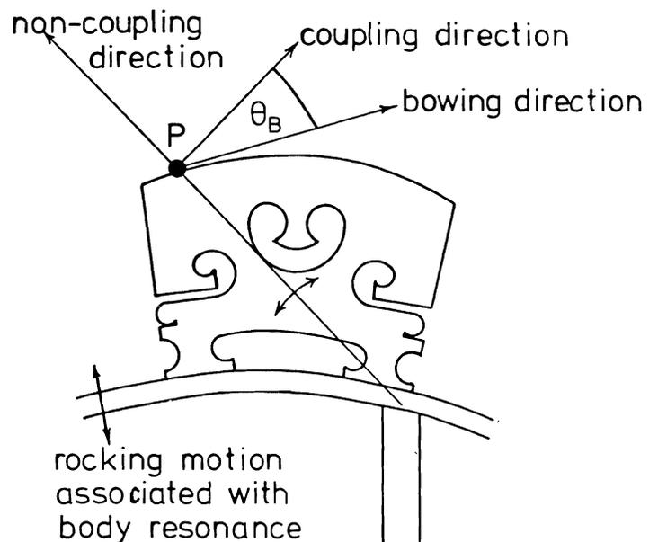
FIG.3: Coupling induced by string vibrations near main body resonance
