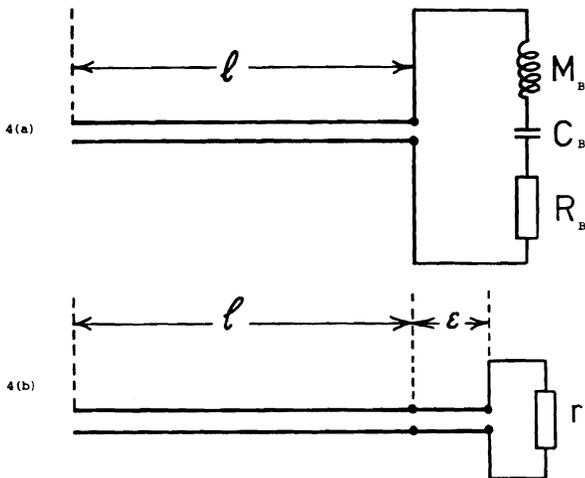
FIG.4(a): Transmission line analogue of string coupled to a structural resonance
