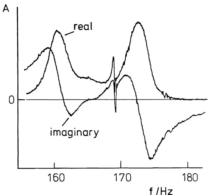
FIG.7:  $n=2$  resonance of a cello C-string in neighbourhood of a strongly coupled main body resonance
